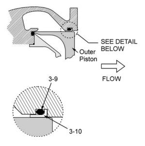
Outer Piston Seal Installation FIGURE 6
