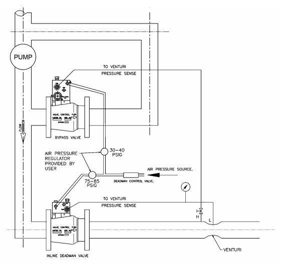
NOTE: THE INLINE AND BYPASS VALVES SHALL BE INSTALLED IN SUCH WAY THAT THE PRESSURE SENSE PORTS SHALL BE LOCATED IN THE TOP POSITION OF BOTH VALVES TO ACHIEVE SATISFACTORY BLEEDING OF TRAPPED AIR.
