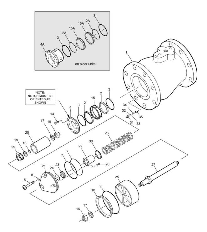
FIGURE 4 47511-1 4" Valve Assembly Used on 64510
