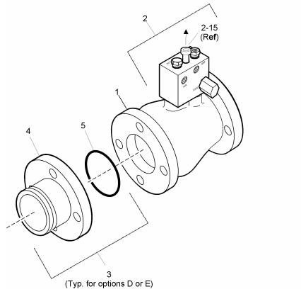
FIGURE 1 – INLINE VALVE ILLUSTRATION
