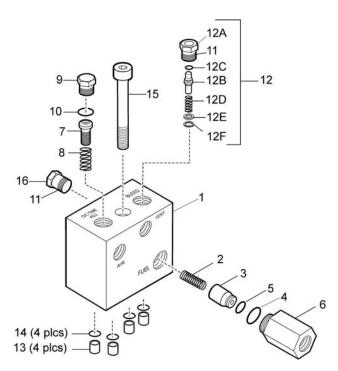
Figure 2 Manifold Parts Breakdown
